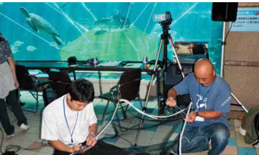
Workshop participants collaborate to modify the prototype for a pound net escape device (PED) as part of experimental trials in Kobe, Japan. © SEA TURTLE ASSOCIATION OF JAPAN. AT RIGHT: A loggerhead turtle successfully escapes a model pound net trap through a prototype PED inside the exhibition tank of Suma Aqualife Park in Kobe, Japan. During experimental trials, several PED designs that ensured both turtle escape and target fish retention were developed. Field trials are planned for 2012–2013. PHOTO: THE YOMIURI SHIMBUN
